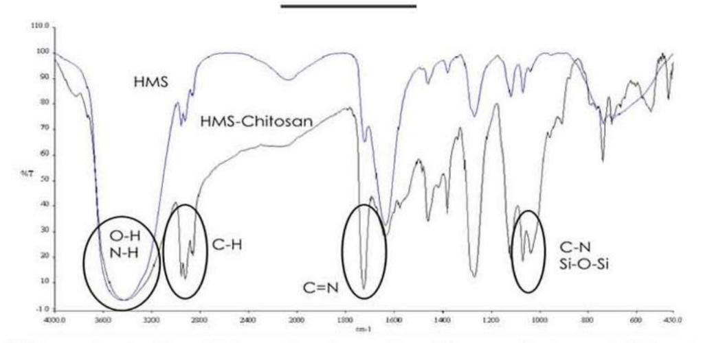
FT-IR analysis. The FT-IR spectra shows the difference between HMS and HMS-chitosan. Bonds such as C=N, Si-O-Si, C-N, C-H can be seen more significantly on HMS-chitosan. This shows the result of the functionalization of HMS using 3-APTES, glutaraldehyde and chitosan.
