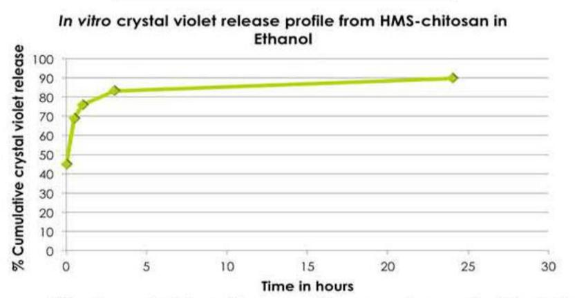
Release profile. Crystal violet release profile was taken at 0, 1/2, 1, 3 and 24 hour intervals. The results showed that at 24-hour interval, the cumulative release of crystal violet is 89.7%. This may suggests that the release of crystal violet from HMS-chitosan is a sustainable one.
