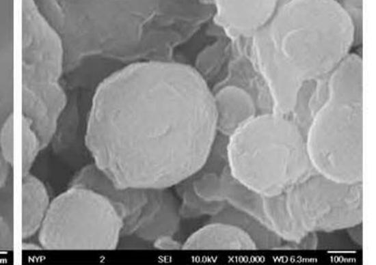
FE-SEM analysis. HMS (left image) and HMS-chitosan (right image) topology at x100,000 magnification. The topology of HMS shows that the unmodified nanomaterial have pores on the surface whereas the topology of HMSchitosan shows a layer of modification to the surface of the nanomaterial upon the addition of 3-APTES, glutaraldehyde and chitosan.
